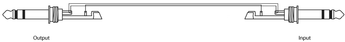
Cable to balanced input from balanced output. TRS connectors.
